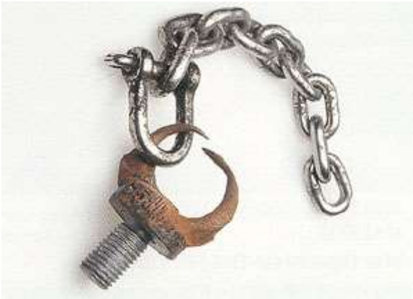
Galvanic corrosion of eye bolt connected to a stainless
