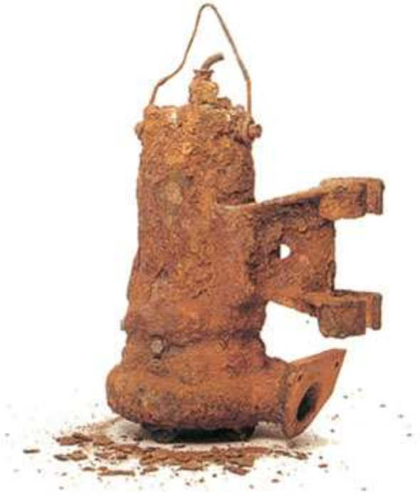
General corrosion on a competitor's cast iron pump.
