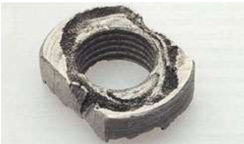
Crevice corrosion on a stainless steel nut exposed to seawater.
