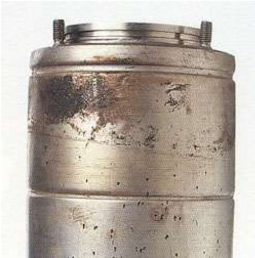
Pitting corrosion on a stainless steel stator housing operating in seawater.
