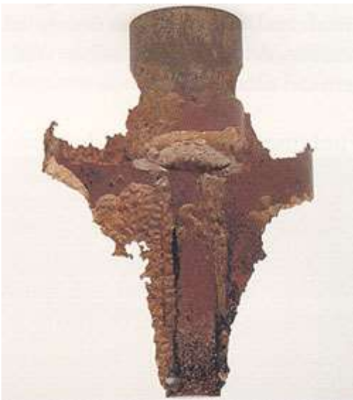
Erosion corrosion on an impeller.
