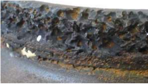
Cavitation corrosion on an impeller.
