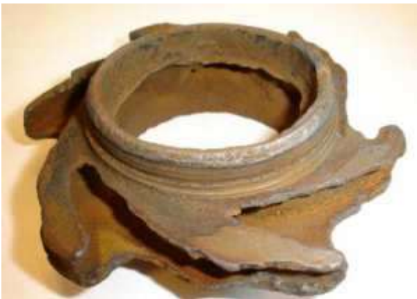
Graphitic corrosion of an impeller made of grey cast iron.
